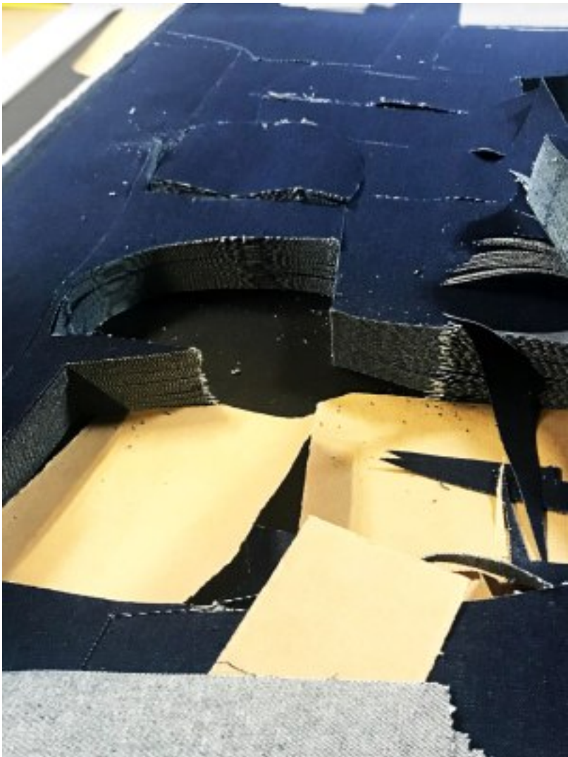
The demo revealed capacity for cutting up to 67 ply of denim. Kaley Roshitsh/WWD
